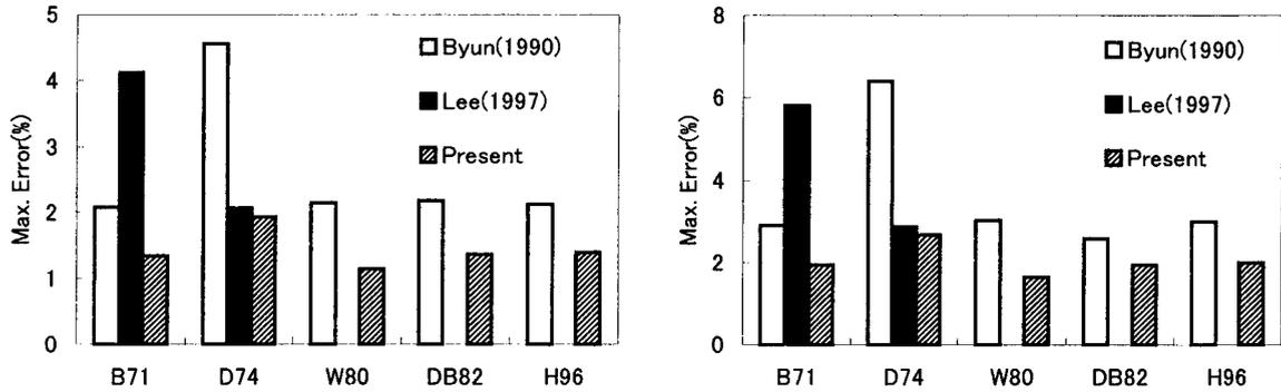
FIG. 4. The maximum errors (%) of (left) drag coefficient and (right) heat exchange coefficient of three analytical solutions for  $z_0 = z_T$ . The abbreviations are defined in Table 1.
