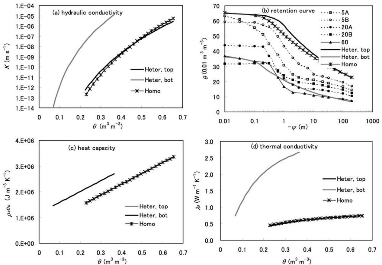
**Figure 5.** Comparison of soil hydraulic and thermal functions between two optimization cases (heterogeneous case and homogeneous case) for the GAME-Tibet Anduo site, 1998. Retention curves analyzed from five soil samples (see Table 4) are also plotted in Figure 5b to compare with the optimized curves. Heter, heterogeneous case; Homo, homogeneous case; top, topsoil domain; bot, bottom soil domain. In Figures 5c and 5d, the curves for the “Heter, bot” and “Homo” fall on top of each other.
