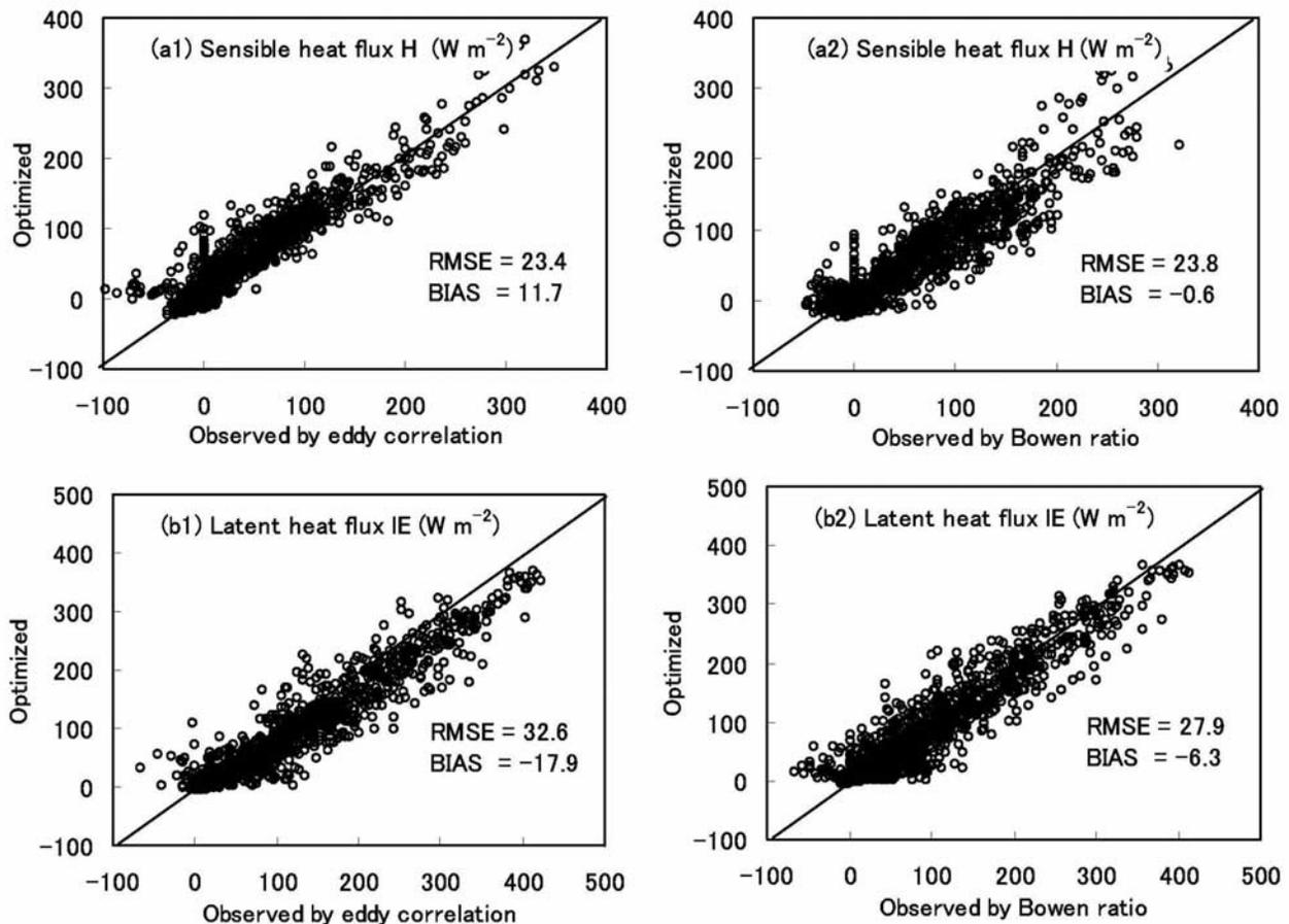
**Figure 8.** Comparison of sensible heat flux and latent heat flux between the observations and the optimized values (from the inverse calibration) for the heterogeneous case of the GAME-Tibet Anduo site during 16 June to 30 August 1998. The root mean square error and bias are indicated for each variable.
