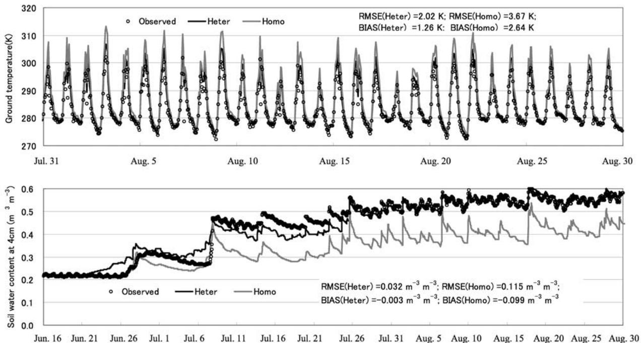
**Figure 7.** Comparison of ground temperature (plotted only for August to save space) and near-surface (4 cm) soil moisture (all the data are plotted) between the observations, the heterogeneous case (“Heter”), and the homogeneous case (“Homo”) for the GAME-Tibet Anduo site, 1998.
