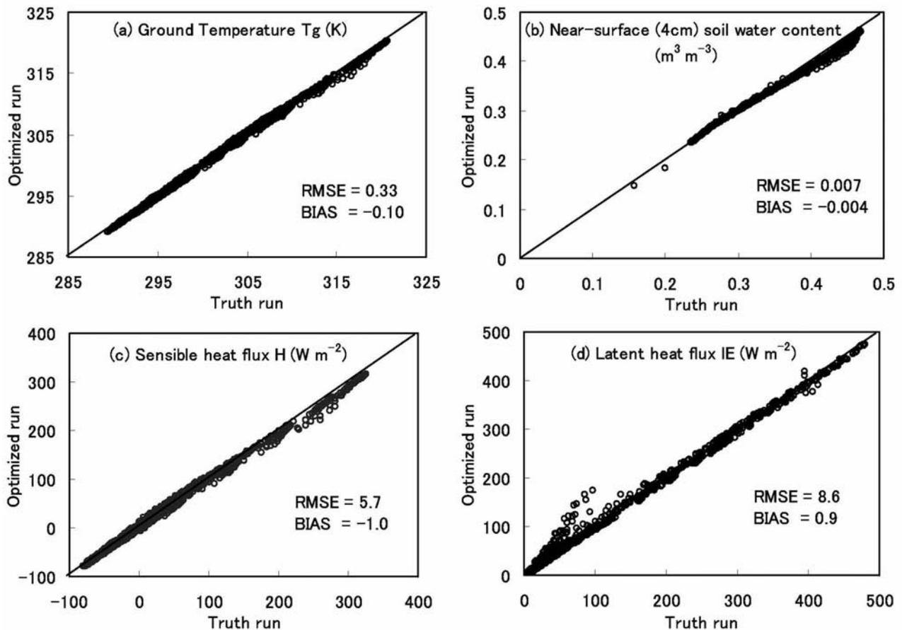
**Figure 3.** Comparison of ground temperature, near-surface soil moisture, sensible heat flux, and latent heat flux between the “true” values (from the forward run) and the optimized values (from the inverse calibration) for the heterogeneous case of the identical twin study. The root mean square error and bias are indicated for each variable.
