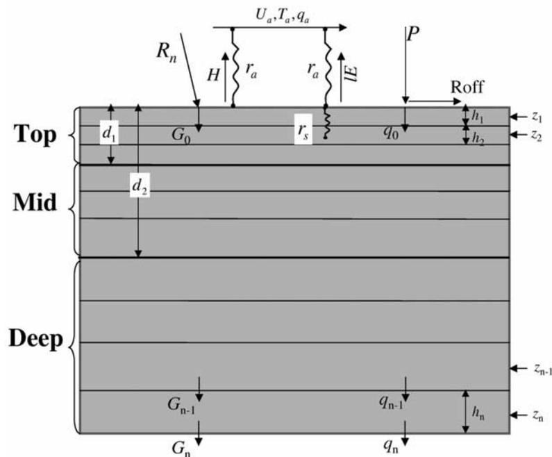
**Figure 1.** Schematic of the single-source land surface model used in this study. There are three soil domains (Top, Mid, Deep), each of which contains multiple computational layers. All the symbols have their common meanings.
