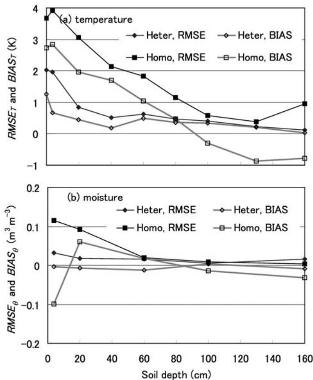
**Figure 6.** (a) Root mean square errors (RMSE) and biased errors (BIAS) of soil temperature at nine measuring depths and (b) soil moisture at five measuring levels for the heterogeneous case (“Heter”) and the homogeneous case (“Homo”) for the GAME-Tibet Anduo site during 16 June to 30 August 1998.
