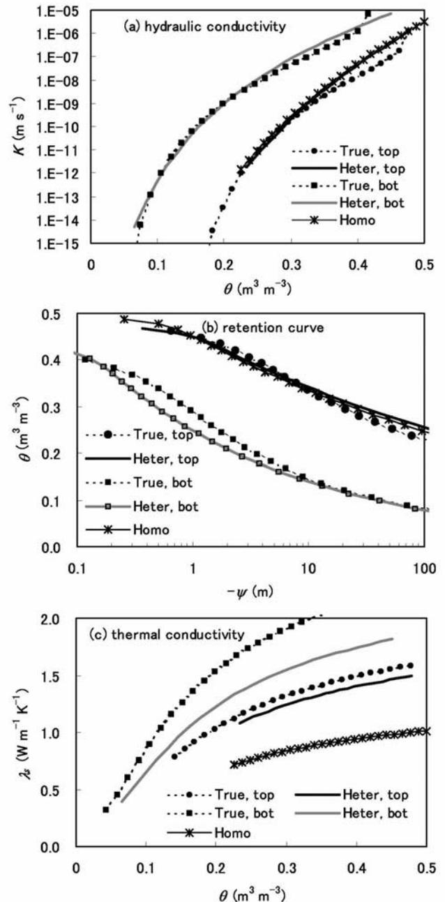
**Figure 2.** Comparison of soil hydraulic and thermal functions (for both the topsoil domain and the bottom soil domain) between the forward run and the optimized run of the identical twin study. Both the heterogeneous case (“Heter”) and homogeneous case (“Homo”) are shown.
